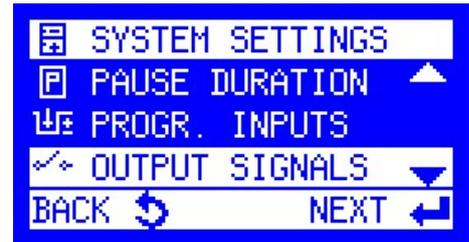
With the option "I/O extension board" further 5 freely configurable output signals are available.
