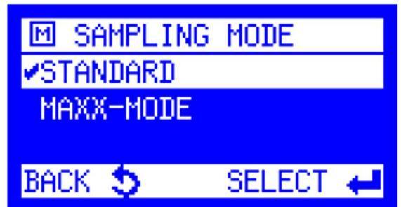
„**MAXX-MODE**“: This function now enables sampling depending on the sensor status. If one of the sensors doesn't longer detecting water (medium) correctly due to contamination in the hose, this mode is automatically switched to and "missing" values from the sensors are replaced by existing, saved values. A calibration must also have been carried out here beforehand.
