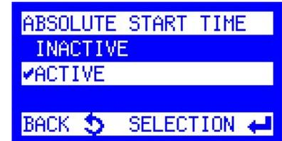
The program is automatically stopped after the entered run time (here: 24 h) and waits for the next external pulse (e.g. by means of a palm button).
