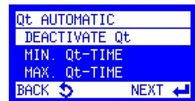
This function enables that in the flow mode (**independently** of the flow signal) a sample is extracted at least after xxx minutes or at the earliest after xxx minutes. Both functions can be activated separately or together.
