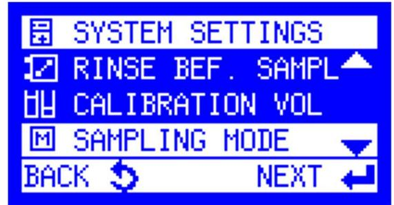
„**STANDARD**“: the sample volume is determined by the two sensors. The system must be calibrated beforehand (ideally at the measuring point).
