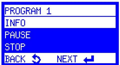
After selection of INFO all details regarding the running program are shown. The single screens can be displayed by pressing the up/down arrow keys.
