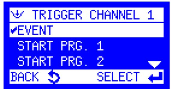
After you have configured **TRIGGER(CH) 1**, it appears the menu already with the real measured value from your sensor. (if it appears "LIMIT VALUE ", it means an exceeded setpoint).
